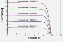
I-V CURVES OF PV MODULE(530W)
